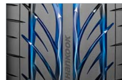
Y-shape pattern Improved water drainage
